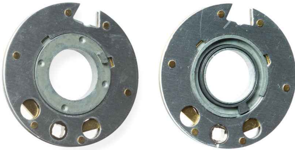
Figure 5: Wheels (front and back). Left : Front; note the drive pin protruding near the axis. Right : Back; note the fly near the axis, which mates with the adjacent wheel's drive pin. This wheel (for a Kaba-Ilco 673 lock) has a movable fly , designed to rotate within a fixed range before moving the wheel; this allows the same combination number to be dialed either clockwise or counterclockwise.
