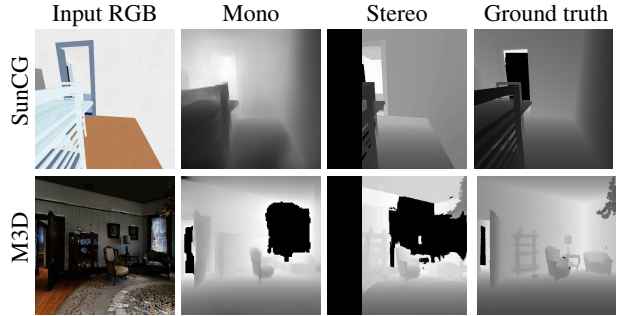
Figure 8. Typical estimated depth maps. Textureless regions and repetitive textures can lead to major errors when using stereo matching (see for instance wall n the top row). Even if the global structure is correct, metric imprecisions in depth estimation lead to drift of the SLAM system.
