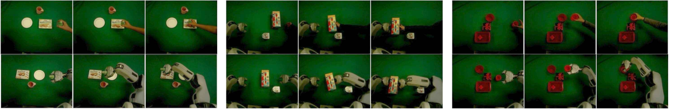
Fig. 5. Example placing (left), pushing (middle), and pick-and-place (right) tasks, from the robot’s perspective. The top row shows the human demonstrations used in Section VI-A, while the bottom shows the robot demonstration.
