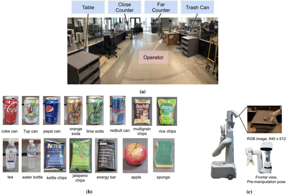
Figure 8: The experiments were performed in a mock office kitchen mirroring this setup (a), with 5 predicted locations and 15 objects (b). The robot is a mobile manipulator with a 7 degree-of-freedom arm and a gripper with policies trained from an RGB observation (c).
