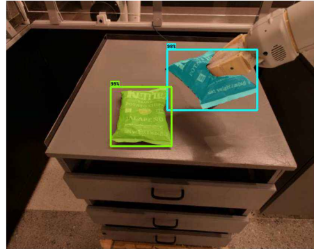
Figure 6: An example of ViLD object detection segmentation mask and bounding box predictions.
