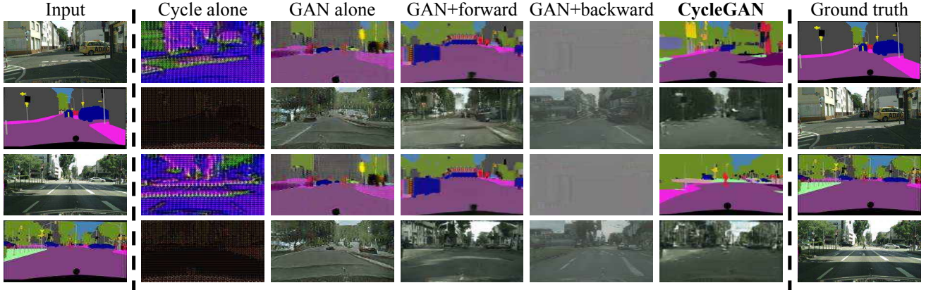
Figure 7: Different variants of our method for mapping labels \leftrightarrow photos trained on cityscapes. From left to right: input, cycle-consistency loss alone, adversarial loss alone, GAN + forward cycle-consistency loss ( F(G(x)) \approx x ), GAN + backward cycle-consistency loss ( G(F(y)) \approx y ), CycleGAN (our full method), and ground truth. Both Cycle alone and GAN + backward fail to produce images similar to the target domain. GAN alone and GAN + forward suffer from mode collapse, producing identical label maps regardless of the input photo.
