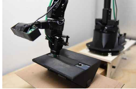
Figure 8: Ethernet cable insertion problem. The automatic reset mechanism changes the position and orientation of the router across tasks.
