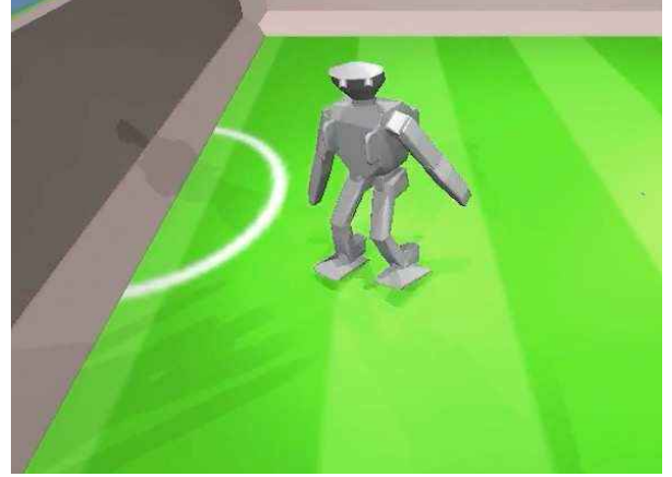
Figure 7 | The OP3 locomotion environment. The 20 DoF humanoid robot can walk around on a plane. The episode terminates early, if the OP3 is about to fall over.
