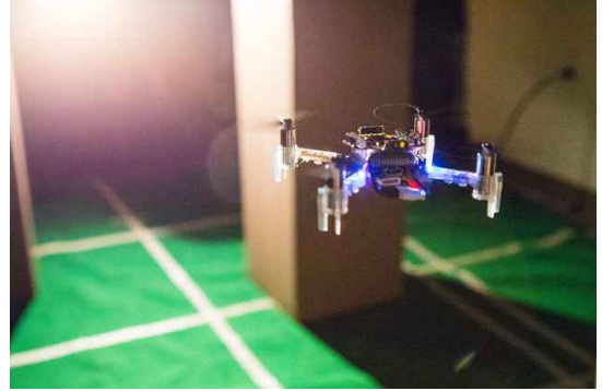
Fig. 1. CrazyFlie nano quadcopter running a deep reinforcement learning policy fully onboard with robust obstacle avoidance and source seeking.
