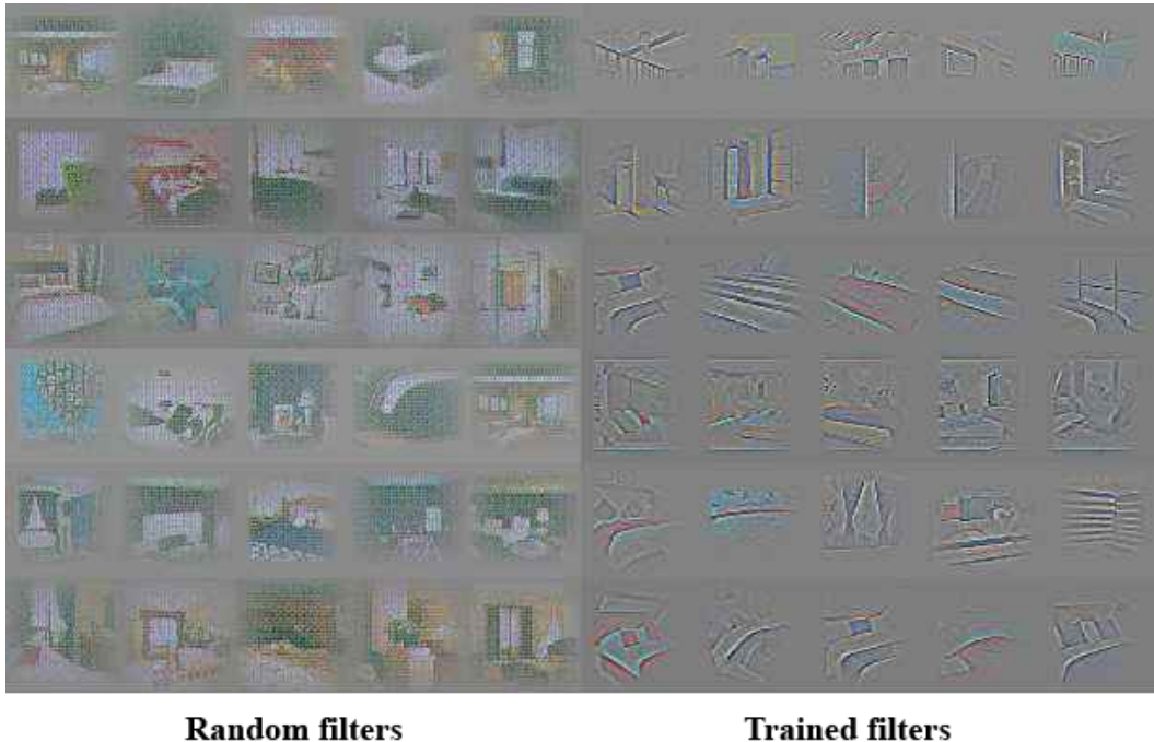
Figure 5: On the right, guided backpropagation visualizations of maximal axis-aligned responses for the first 6 learned convolutional features from the last convolution layer in the discriminator. Notice a significant minority of features respond to beds - the central object in the LSUN bedrooms dataset. On the left is a random filter baseline. Comparing to the previous responses there is little to no discrimination and random structure.
