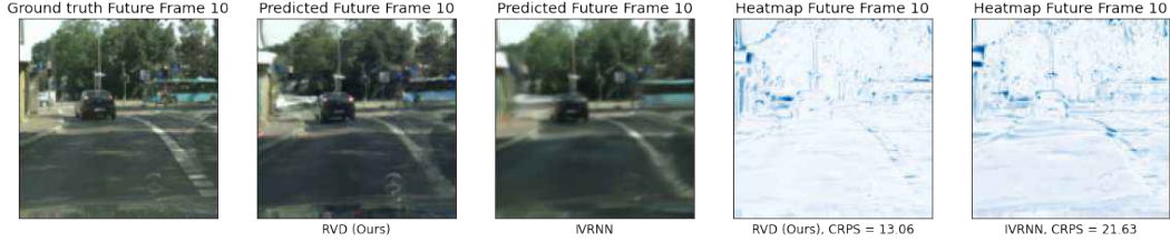
Figure 4: Spatially-resolved CRPS metric (higher is better, see Section 3). We compare the performance of RVD (proposed) against IVRNN on predicting the 10 th future frame of a video from CityScape. The right two images show the spatially-resolved CRPS scores. Darker areas point to larger disagreements. Our model exhibits less disagreement with respect to the ground truth.
