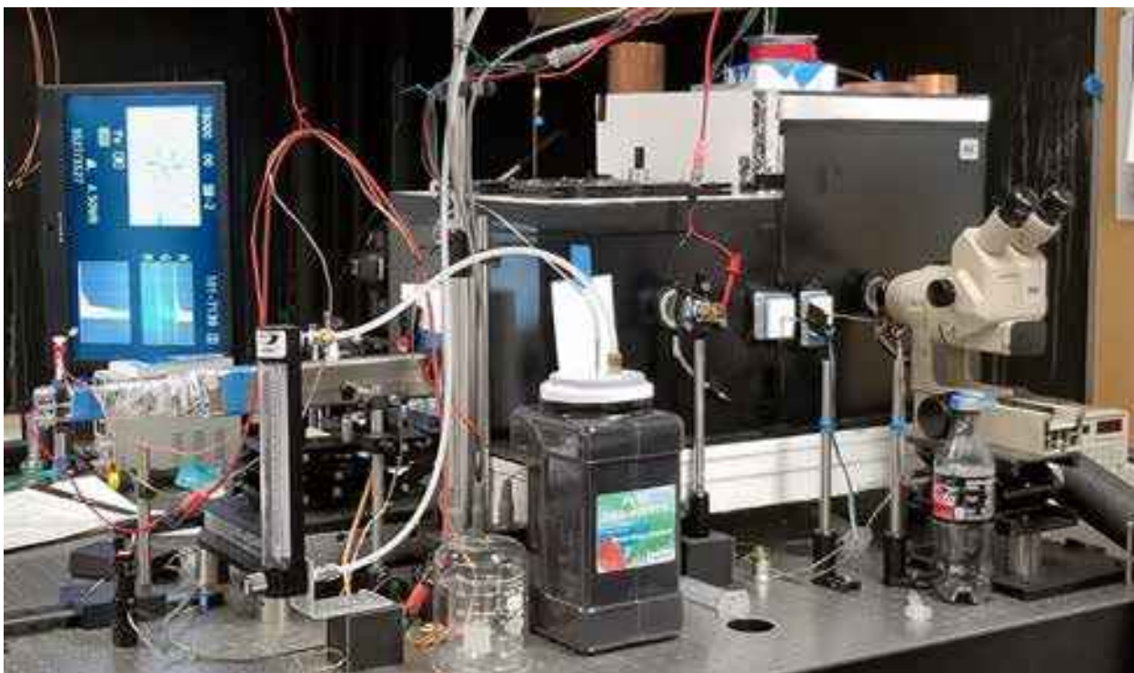
Figure 8.11. A laboratory photograph of the dual diffusion chamber apparatus depicted in Figure 8.10. The recirculating chiller that cools the chambers, as well as several temperature controllers and other pieces of electronic hardware, are not visible in this picture.
