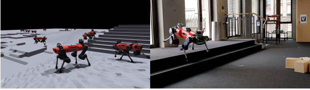
Figure 10: Trained policy for ANYmal on rough terrain tested in simulation and on the real robot.
