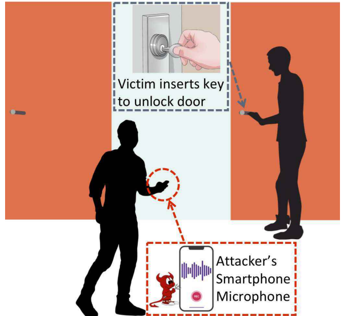
Figure 1: Figure depicts SpiKey attack scenario. Attacker records the sound of victim’s key insertion to infer the shape, or “secret”, of the key.
