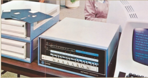
1976: Altair 8800b with 8080A microprocessor, about $5000 with all options and a terminal
