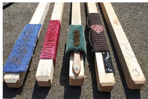
Fig. 1 The tested hair snares (left to right): carpet, rubber band, wire brush, doormat, and wildcat
