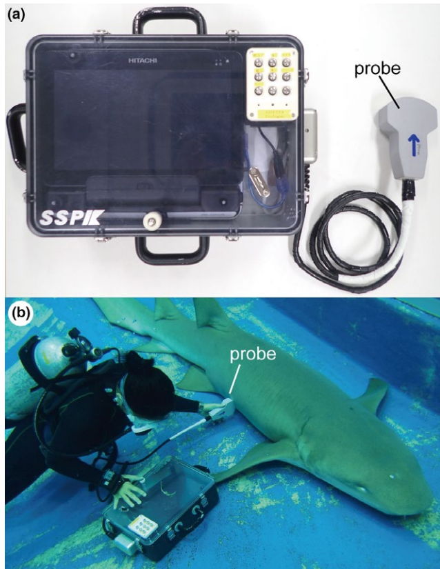
FIGURE 1 Underwater ultrasound developed in this study (a). Ultrasound observation for the pregnant tawny nurse shark at the depth of 10 m in the exhibition tank of Okinawa Churaumi Aquarium (b)
