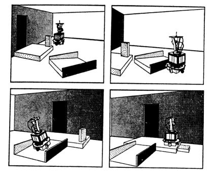
Fig. 9.2 — 'Shakey' in action. The robot is remotely controlled over a radio link.
