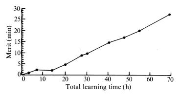
Fig. 16.11 — The pole-and-cart system, set up for pure trial-and-error learning. The lower curve shows a smoothed average ('merit') of the time-until-crash, plotted against the total accumulated learning time.
