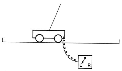
Fig. 14.4 — The pole and cart problem. Chambers and Michie's BOXES program generated a rule-based controller. The controller's task was to keep the pole balanced and the cart on the track.
