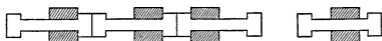
Fig. 20. The buffer, D , attached at the centre of each unit. This device prevents close contact of more than two units which are aligned with one another.
