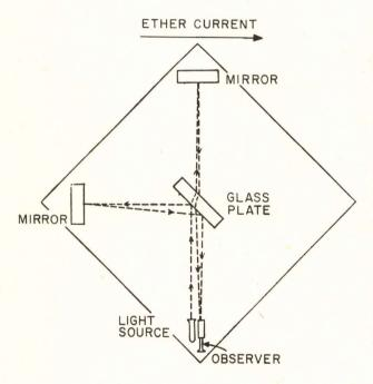
A simplified diagram of the experiment by which Michelson disproved the existence of an "ether drift." The beam from the light source is broken into two beams in opposite directions and brought back to the observer.
