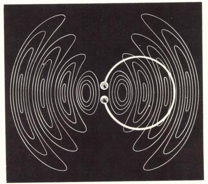
Electromagnetic waves. Hertz discovered that this pattern of waves was produced around an electric spark. The spark is produced in the gap in the ring-shaped object, called a resonator.
