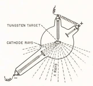
An X-ray tube. When the stream of electrons hits the piece of metal called a target, X-rays are given off.
