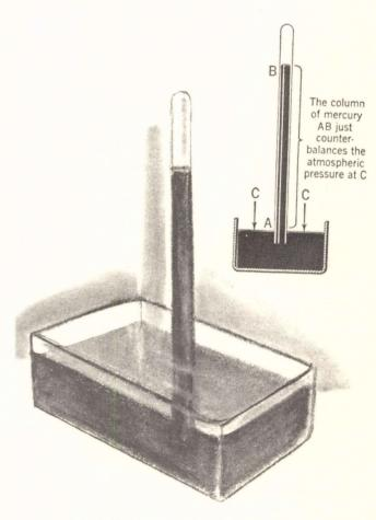
Torricelli's experiment on air pressure.
