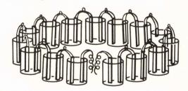
An early battery. After the voltaic pile, the next step was to connect a number of chemical "cells" together. The principle is the same as in the modern automobile battery where a chemical reaction occurs between two metals in a solution called an electrolyte.
