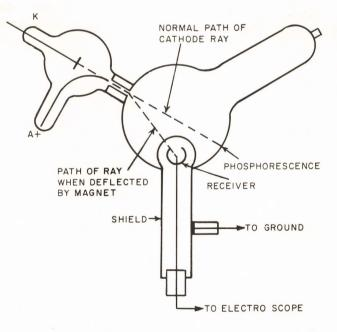
Diagram of how Thomson showed that cathode rays act like electric particles.
