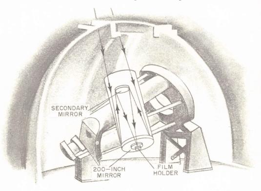
Cutaway view of the giant reflecting telescope on Mount Palomar.
