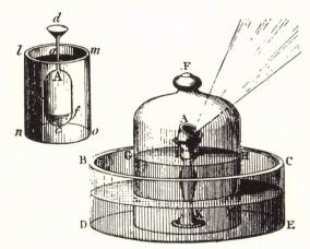
Hydrometer developed by Lavoisier. From a drawing of the time.
