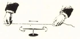
Oersted's experiment. A wire carrying an electric current will cause the magnetic needle to turn.
