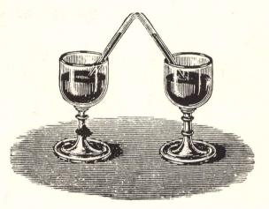
This simple apparatus was used by Cavendish for a very important experiment. With a mixture of oxygen and air in the bent tube, he passed electric sparks through it until all the oxygen and nitrogen had combined, and showed that air is composed almost entirely of these gases.
