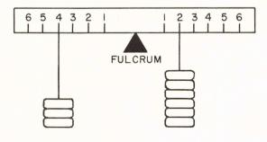
BALANCING A 3 LB. WEIGHT AT 4 FT. WITH A 6 LB. WEIGHT AT 2 FT.
