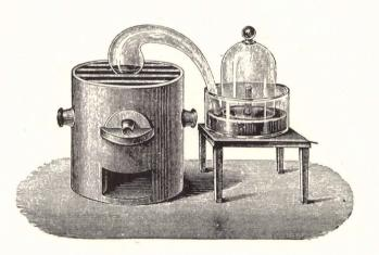
Lavoisier's mercury oxide apparatus. From a drawing of the time.
