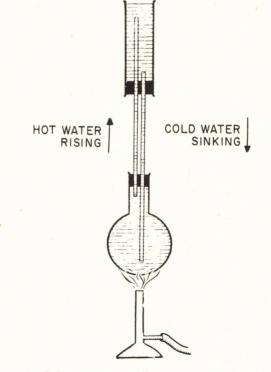
A laboratory model of convection heating, the basic principle of a central heating system.
