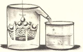
fine way to measure an irregular volume. Archimedes filled a container with water and carefully suspended the suspected crown in the water. He caught the water that spilled out the overflow must be the same volume as the crown. Now it was a simple job: obtain a volume of gold equal to the volume of the water and check its weight against the weight of the crown.
