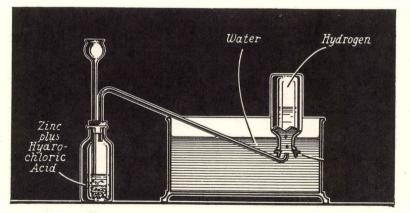
Making hydrogen in the laboratory.
