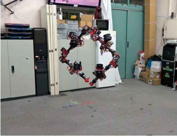
Figure 15. Stable hovering under the challenge configuration by the proposed control method. This configuration is a singularity in the previous control method (Zhao et al., 2021). The related video can be found in https://youtu.be/fJA4Rch0biE .
