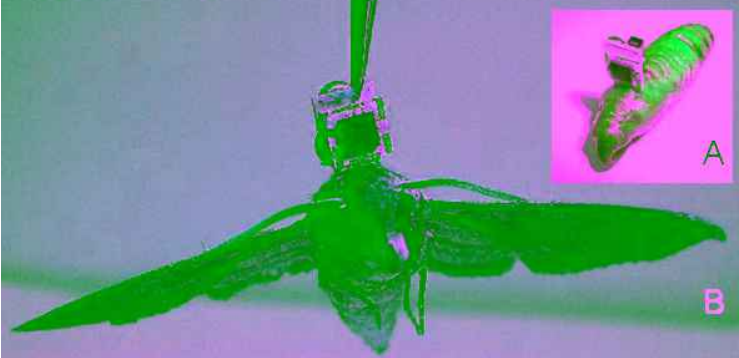
Figure 57: Pupal stage insertion (A) and successful emergence (B). The microsystem platform on (ii) is held with tweezers to show wing opening of the moth.
