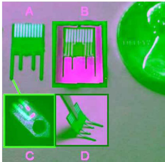
Figure 34: The flexible polyimide probe (A) and silicon probe (B). The close-up view of the tip in (C) with the hole for muscle growth, and the flexibility of the probe (D) are also given.
