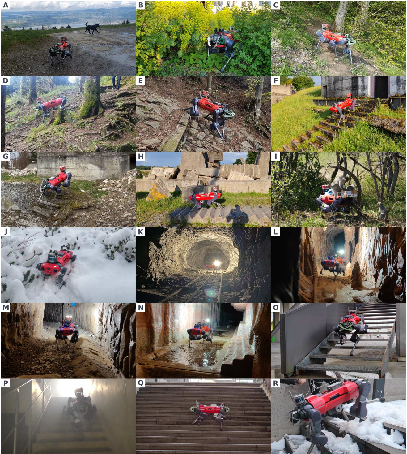
Fig. 1. Robust locomotion in the wild. The presented locomotion controller was extensively tested in a variety of complex environments over multiple seasons. The controller overcame a whole spectrum of real-world challenges, often encountering them in combination. These include slippery surfaces, steep inclinations, complex terrain, and vegetation in natural environments. In search-and-rescue scenarios, the controller dealt with steep stairs, unknown payloads, and perception-degrading fog. Reflective surfaces, loose ground, low light, and water puddles were encountered in underground cave systems. Soft and slippery snow piled up in the winter. The controller traversed these environments with zero failures.
