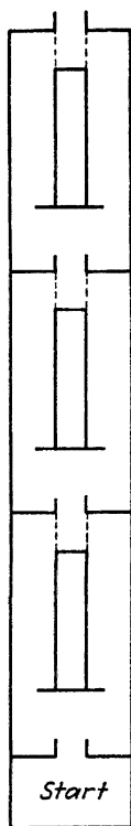
FIG. 83.—Walton's Sectional maze. Any number of units may be placed end to end and either the right or left route through a section may be blocked by inserting a board at any of the points indicated by broken lines. ( Modified from Walton, 1930, p. 55. )
