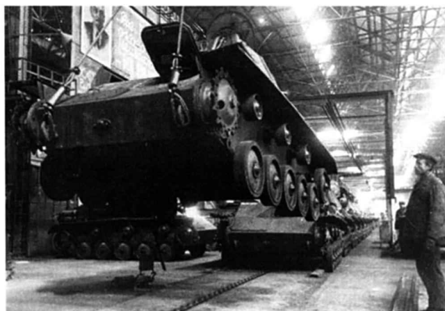
Figure 12. Assembling T-70 tanks at Molotov (Gorky) Automobile Plant, 1942. Photo courtesy of the State Political Archive of the Nizhny Novgorod Region.
