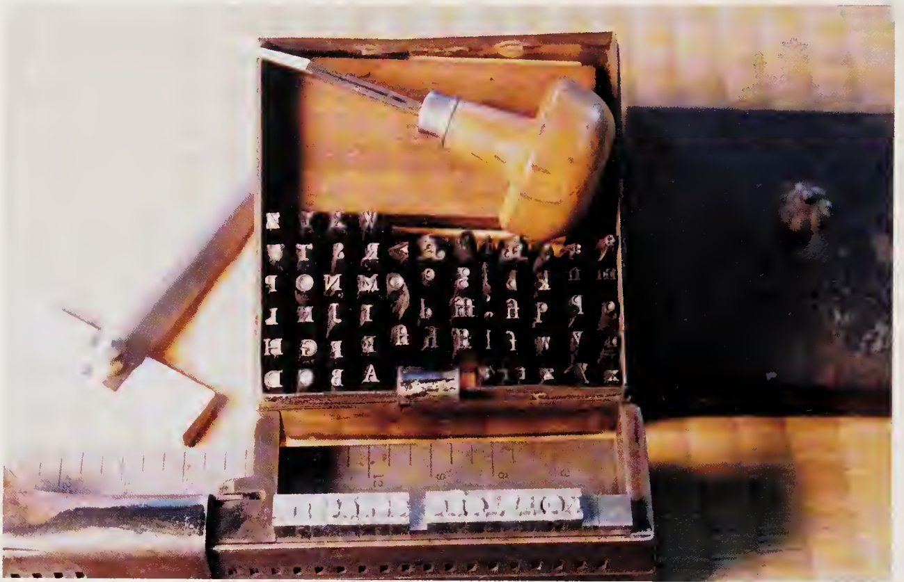
3. Regulus in composing stick with punches and graver.
