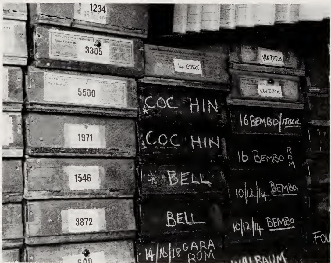
3. The keybars that control the operation of the Monotype keyboard are housed in these wooden boxes, with the name of the fount written on each box
