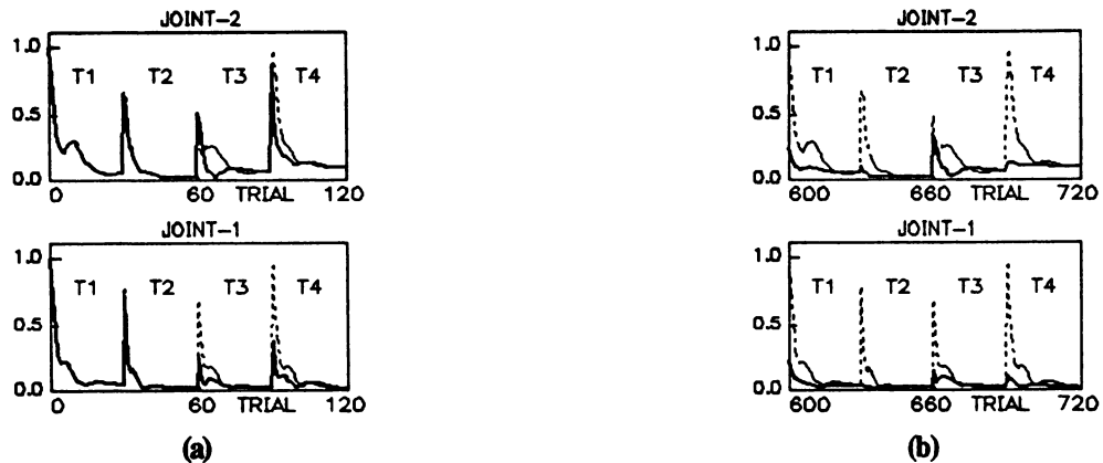
Fig. 5 Curves of normalized RMSE of angle vs. trials showing generalization. Four trajectories (T1-T4) are learned successively.
