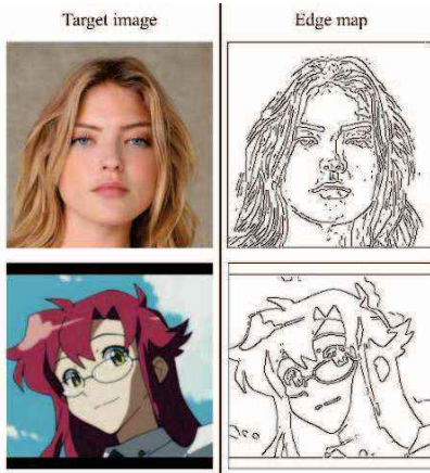
Fig. 2. Edge maps extracted from target images. The thresholds of first and second row are 5, 100 and 12, 100 respectively.
