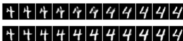
(b) Image generation via linear interpolation of two latent space representations of MNIST digit 4 using a trained Autoencoder (top) and ReGene Classifier (bottom).
