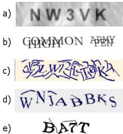
Figure 2: A gallery of text CAPTCHAs. Simple text challenges, such as a (register.com), are still common despite recent defeat by optical character recognition. Researchers have begun to focus on schemes that make letter segmentation difficult, as seen in b (Carnegie Mellon [13]) and c (Microsoft Research [2]). Webmasters, wary of what users will tolerate, dial back researchers’ noise parameters, seen in d (Microsoft Hotmail) and e (Yahoo! Mail).
