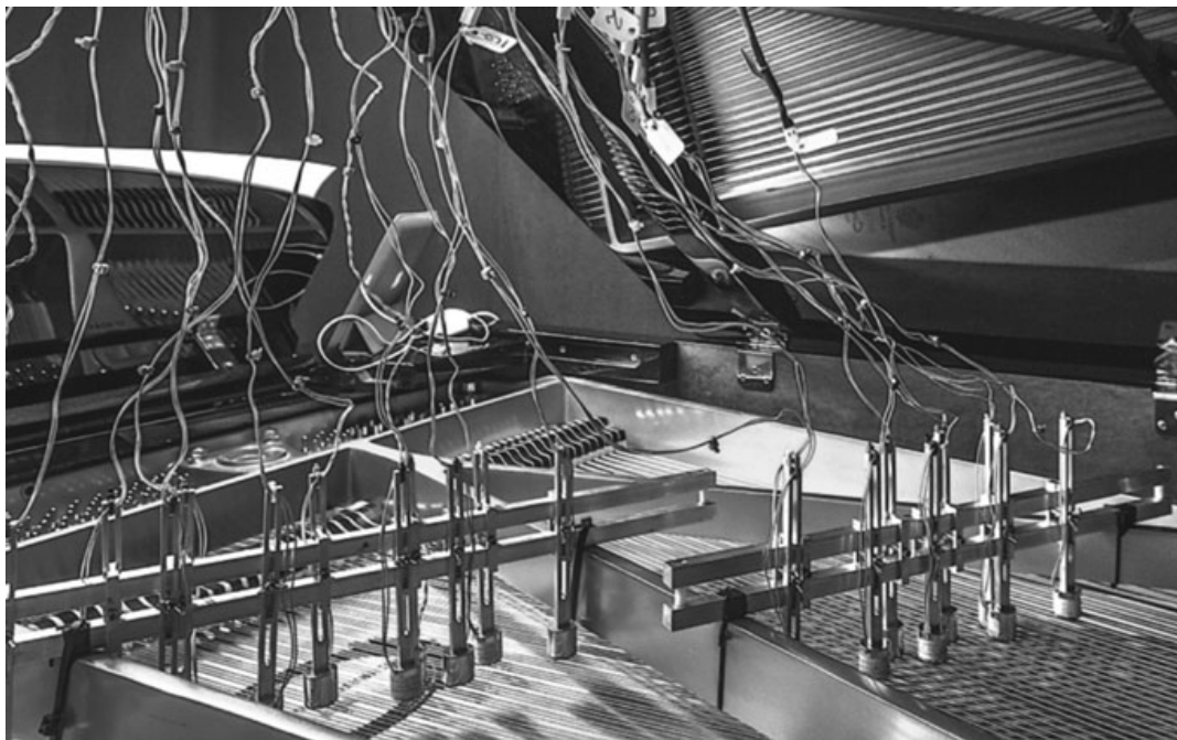
Fig. 14 A photograph of twenty-four electromagnets furnished above the strings of a grand piano
