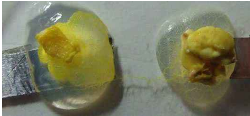
Fig. 3 Photograph of the experimental environment for growing and measuring the electrical properties of 10 mm plasmodial tubes
