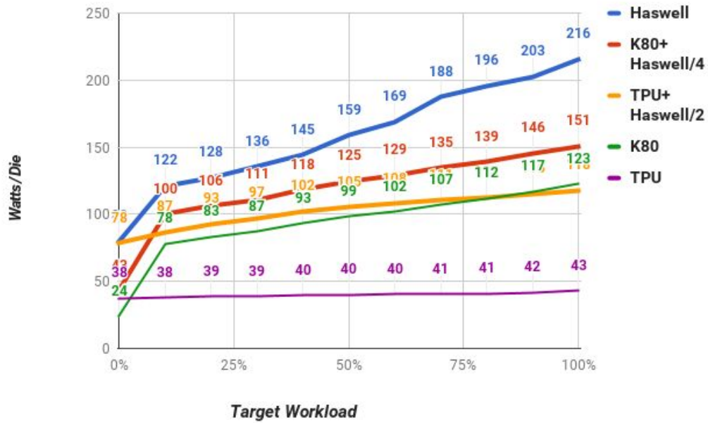
Figure 10. Watts/die for CNN0 as target platform utilization varies from 0% to 100%. The Total GPU and TPU power are the red and orange lines and their Incremental power are the green and purple lines. (The blue line is Haswell, which by definition is total power.) A server has 2 CPUs and 8 GPUs or 4 TPUs, so we normalize power by dividing by 2, 8, and 4, respectively.
