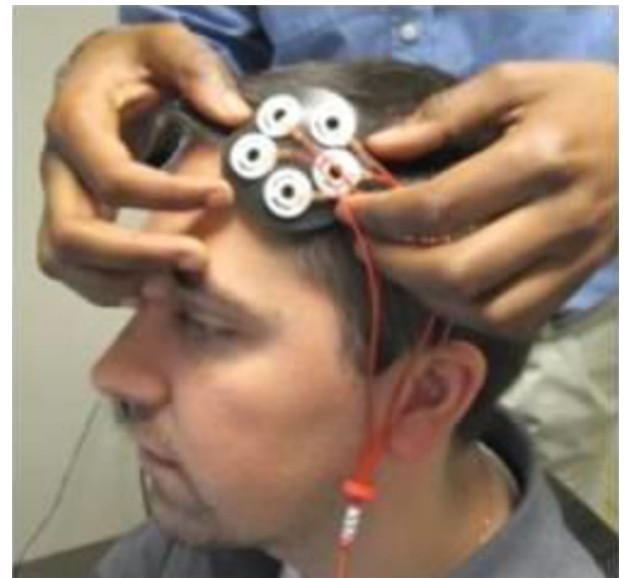
Figure 1. tDCS electrode array (anode only pictured). All five elements are standard silver–silver chloride EEG electrodes placed in a plastic cup which is then filled with a conductive gel.
