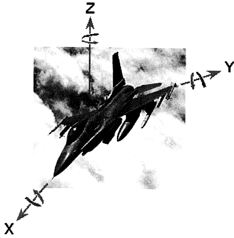
Fig. 10 Major axes between flight motion and flight instruments. (Courtesy of USAF; data available online at http://www.af.mil/photos/fighters .)
