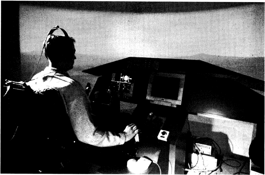
Fig. 5 Laboratory setup for experiments on three-dimensional audio in the cockpit. Note the head tracker on the headphones.
