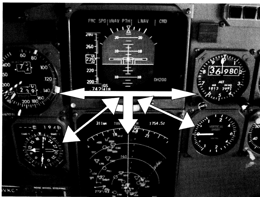
Fig. 9 Arrows illustrate the typical instrument cross-check pattern with individual instruments. Depending upon the flight task, the frequency and dwell time on each display can vary.
