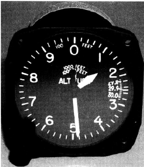
Fig. 5 Typical mechanical altimeter with barometric pressure setting window at the three o'clock position. Large white pointer indicates hundreds, and small white pointer indicates thousands. A ten-thousands pointer can be seen in some altimeters, as well as warning stripes for low altitude (usually below 10,000 ft). (Courtesy of NASA Ames Research Center, Moffett Field, California.)
