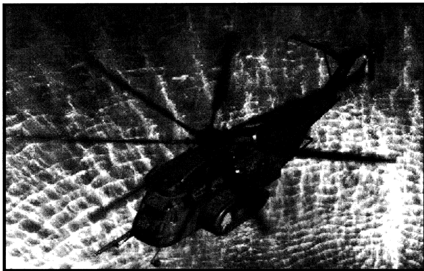
Fig. 7 Illustration of the linear motion stimulus created by the rotor wash of a helicopter. (Photo reproduced with permission of Art Estrada.)
