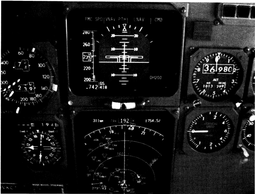
Fig. 13 Typical arrangement of the flight instruments emphasizing the central location of the attitude indicator.
