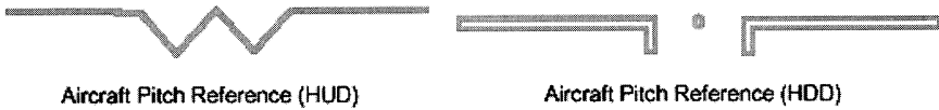
Fig. 17 Two miniature aircraft symbols commonly used for the attitude indicator pitch reference. The term “miniature aircraft symbol” has been used to identify any of the symbologies used to depict the aircraft pitch angle and is often termed the pitch reference symbol.
