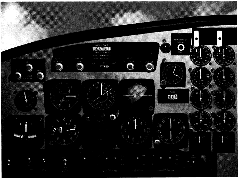
Fig. 7 Representative grouping of control and performance displays (although not the most ideal arrangement). (Courtesy of General Dynamics Advanced Information Systems.)
