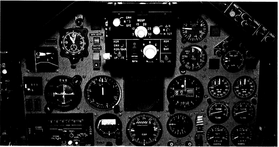
Fig. 1 Low-tech, fighter-type cockpit instrument panel comprised of many head-down displays from which the pilot contrives a mental view of the world of forces, commands, and information. A single display is used to present one particular type of flight data. (Photo courtesy of Gateway and Kaiser Electronics.)
