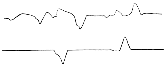
Figure 8.6. Records of two different types of response in attempting to move a pointer on to a target by means of a velocity control. The records are plots against the time (from left to right) of the movements of the control. The upper record shows a normal skilful response with a movement of the control to get the pointer going and a second movement to stop it. The lower record shows a disorganised response made in the attempt to achieve the same result. Data from Davis (1949).
