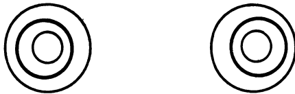
Figure 6.10. If the right-hand circles are viewed by the right eye and the left-hand circles by the left eye in a stereoscope, the outer circles will appear nearer and the middle circles farther away than the centre circles.
