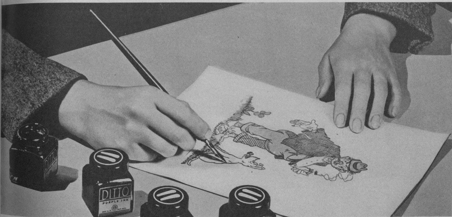
In one operation Ditto's gelatin machine will reproduce eight colors. These colored inks are laid down on a master copy with pen or water color brush.
