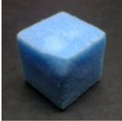
Figure 5.10: 4cm cube of blue styrene foam, aviation grade. Displaying a depressed corner and finger print.
