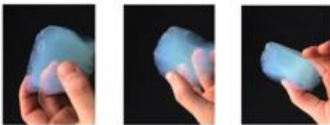
Picture Caption: Silica Aerogel produced by Steven M. Jones of the NASA Jet Propulsion Laboratory. Demonstrated by Zee Loughlin at the Materials Library's Supernatural Materials event at Tate Modern, November 2005.
