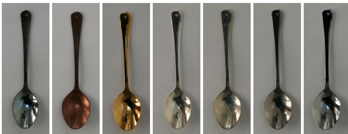
Figure 8.1: From left to right: zinc, copper, gold, silver, tin, stainless steel and chrome.
