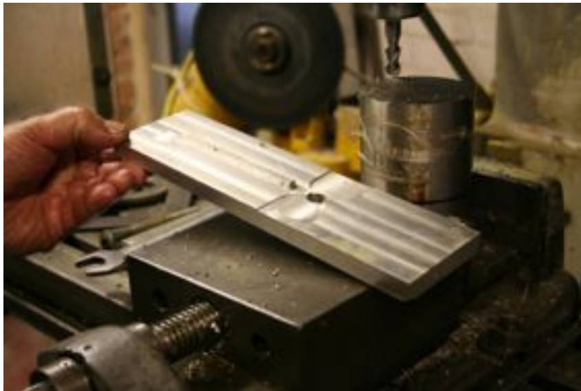
Figure 6.3: Rex Garrod in his workshop showing the jig he made for machining tuning forks.
