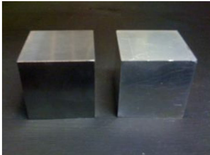
Figure 5.2: The 4cm cubes of tungsten (left) and aluminium (right).
