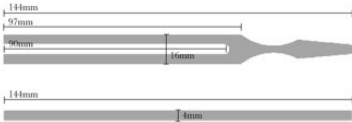
Figure 6.2: An image of the computer-aided design model of the John Walker 440Hz tuning fork generated to be an instruction for digitised manufacturing processes.
