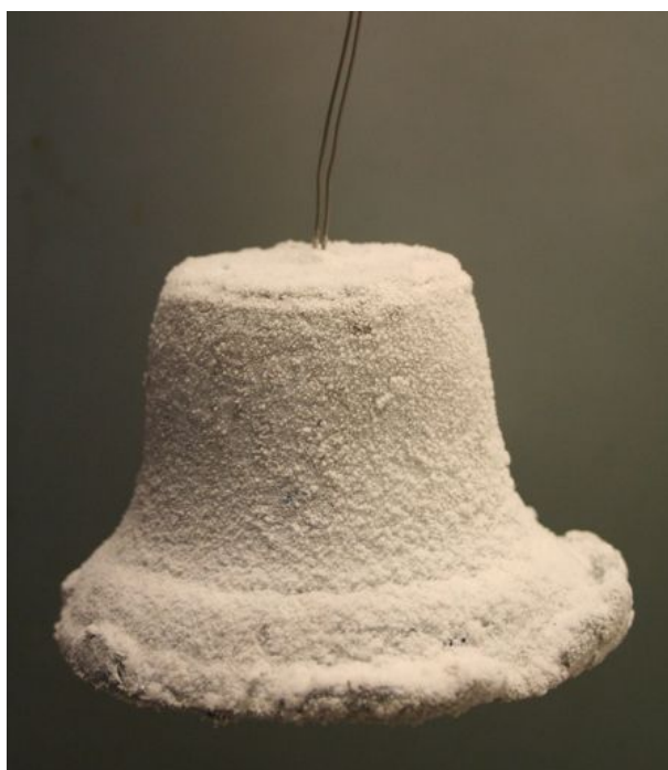
Figure 7.3: The mercury bell made by Dr Andrea Sella of the UCL Chemistry Department. It is required that this bell is stored in a deep freezer at -80^{\circ}\text{C} in order to maintain its solid form. Due to the extremely cold temperature of the material, ice crystals form on the surface of the bell each time it comes into contact with room temperature air, as can be seen in this photograph.
