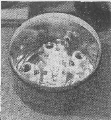
One coffee can plus six small ceramic sockets and a supply of Christmas tree bulbs make a low-energy stove for maintaining solution temperatures.
