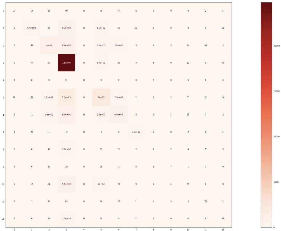
Figure 40: Confusion matrix obtained from results of logistic regression trained on imbalanced dataset formed using Doc2Vec
