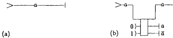
Fig. 22. The value a carried by an arbitrary line (a) can be inspected in a nondestructive way by the “spy” device in (b).
